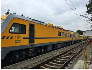
Fig. 12. XLN4C-01 inspection vehicle.
